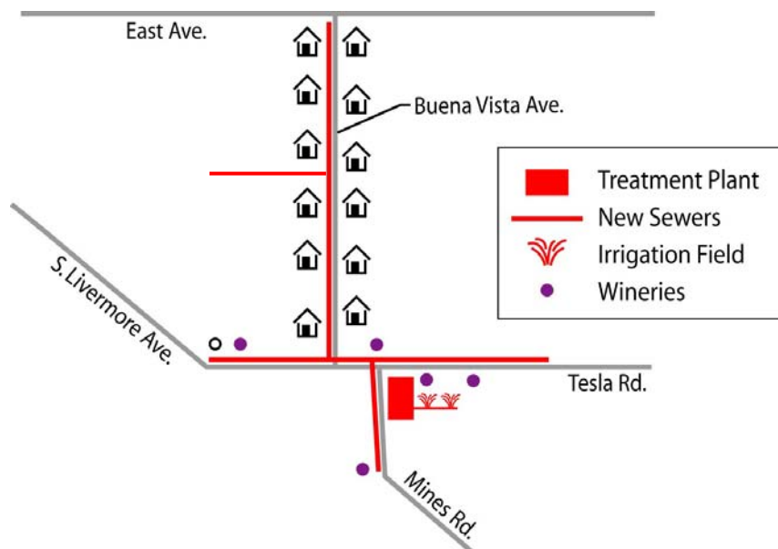
Figure 4 Conceptual Layout of Community Treatment System
